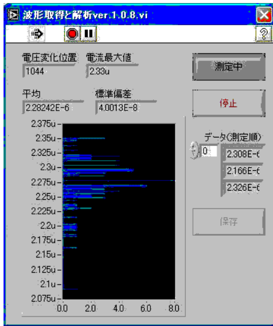
Fig. 10. The electrical signal from the amplifiers are collected by a digital oscilloscope and the data are monitored and stored by a LabView Program.
