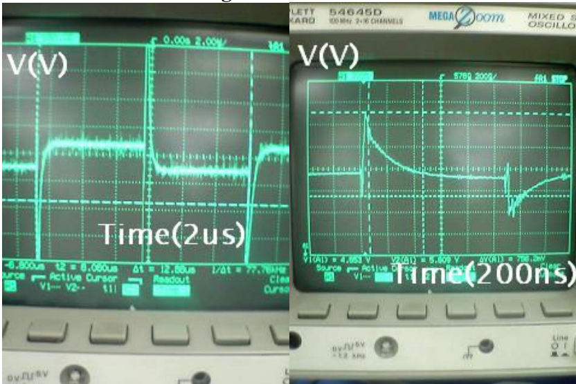
Figure 2.5-1 (left) n of 127-128 oscillating. The period measured as 12.86us as shown on the picture. Figure 2.5-2 (right) n of 127-128 enlarged for amplitude measurement. Vpp of 756.2mV was shown.
