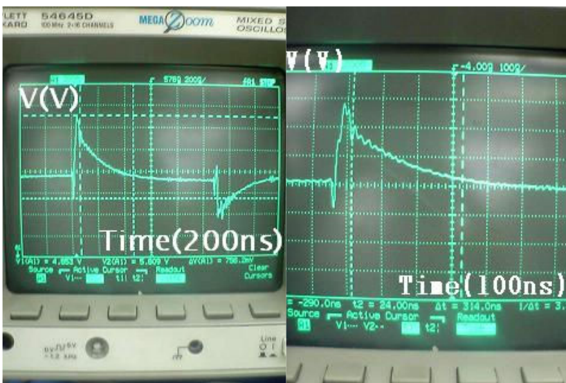
Figure 2.5-3 (left) Measuring Settling Time Figure 2.5-4 (right) Measuring Settling Time in enlarged plot
